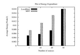
**Figure 12.** Plot of Average Energy Utilization per node (at the end of 150s) for MST and LocalHeur for 100 nodes and 1,10,20,30 sources.
